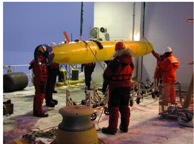
Fig. 2. AUV recovery onboard USCGC Healy October 2001 (photo by Todd Walsh, ©MBARI)
