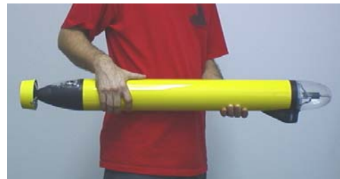
Figure 2: Ranger is a 9cm hull UUV. It uses a stern-mounted, two-axis vectored-thruster for propulsion and control; otherwise it has no fins. Ranger is passively stable in pitch and roll, and trimmed to have slightly positive buoyancy. Ranger comes equipped with CTD sensors, and can accept up to three additional environmental sensors.
