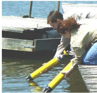
Figure 3: A 2-Ranger launch. Because of its light weight, robustness, and processing power, Ranger is well suited to multi-vehicle applications.
