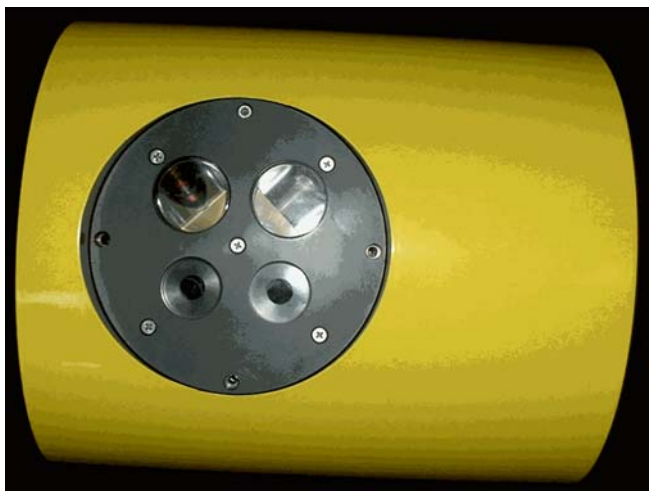
Fig. 3. Hydroscat-2 mounted in the science payload section of the Glider.
