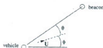
Fig. 4. Vehicle angle \phi and \theta used in stability analysis.
