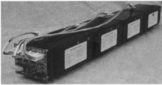
Fig. 8. A 1000-Wh lithium ion pack with smart battery bus interface.
