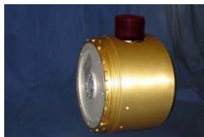
Figure 16 Acoustic communication module
