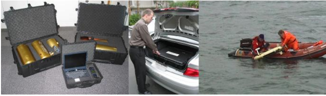
Figure 2 The Gavia Base Vehicle is transported in two Pelican cases with the surface equipment contained in a third smaller case.
