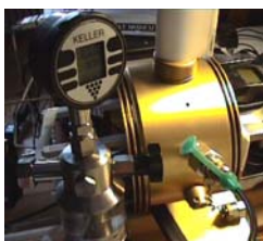
Figure 23 Pressure calibrator screwed into the pressure port of Gavia.
