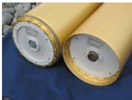
Figure 1 The Gavia modules are splash-proof, facilitating, for example, on-deck Battery Module swapping. The male and female parts of the Gavia modules are shown.
