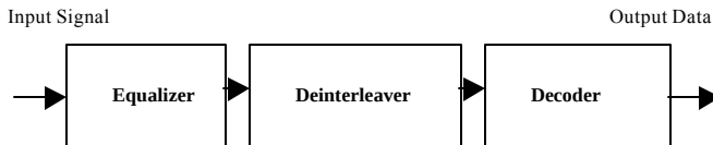
Figure 2. General Acoustic Telemetry Receiver Structure
