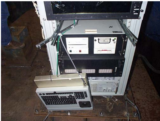
Fig. 10. Keyboard hanging from the broken slider.
