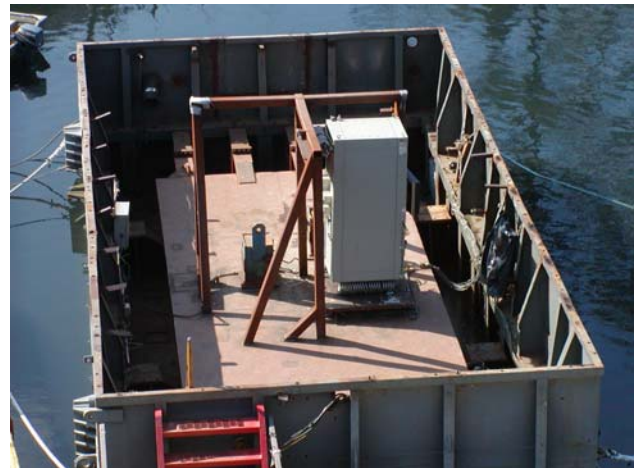
Fig. 6. Pictorial view of the NAVSSI rack under test. The rack was installed in a Floating Shock Platform (FSP) on Deck Simulator fixture
