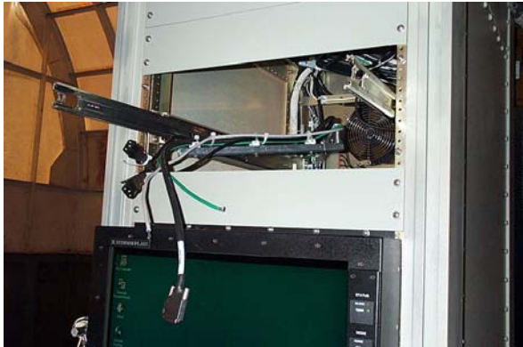
Fig. 9 DCS RAID Drive assembly missing and out of the rack. Pieces of the raid drives were found on the FSP deck.
