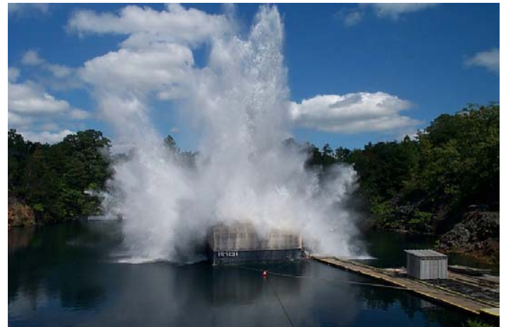
Fig. 8. A Barge Test shot at HI-TEST Laboratories, Inc.
