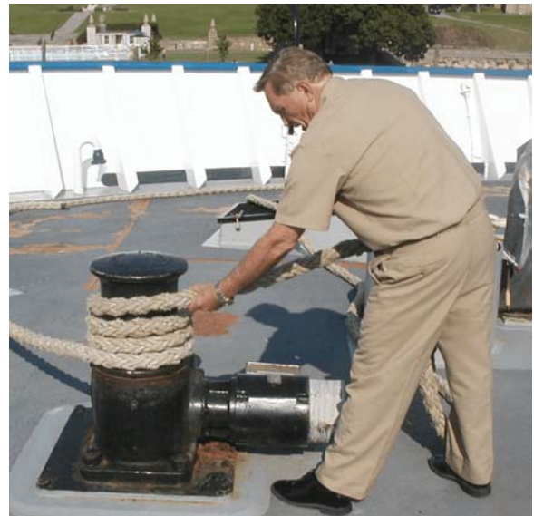
Figure 5 Bad Practice, Too Close and In Rope Path
