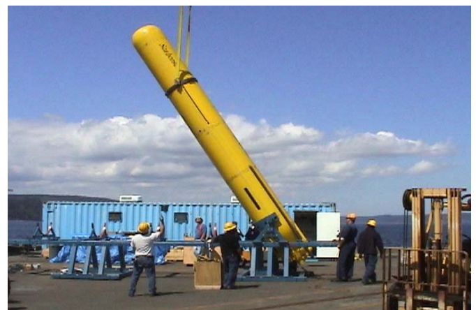
Figure 3. Seahorse being lifted for insertion into launch apparatus
