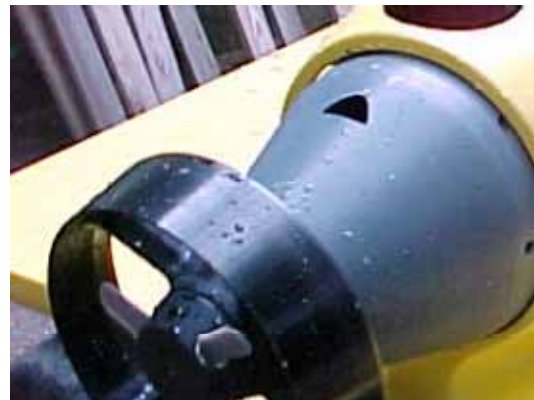
Fig 6. SAUV II Vectored Thruster w/3 Bladed Propeller
