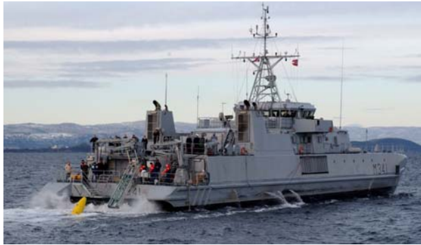
Fig. 2. HUGIN I immediately after launch from the RNoN mine hunter KNM Karmøy in December 2001
