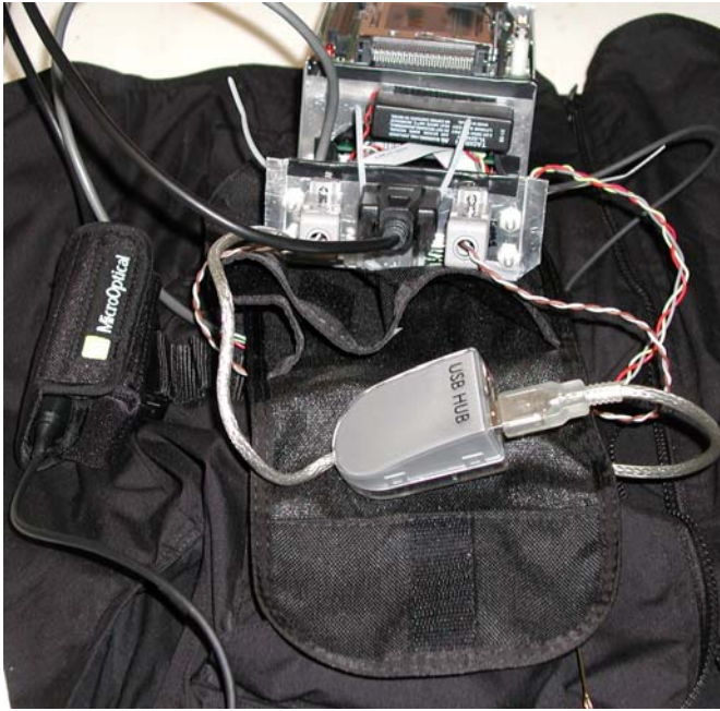
FIGURE 6 PC/104 BOX AND JUNCTION PLATE
