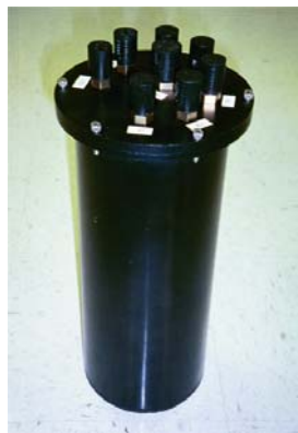
Fig. 7: AUV pressure vessel (1 of 4)
