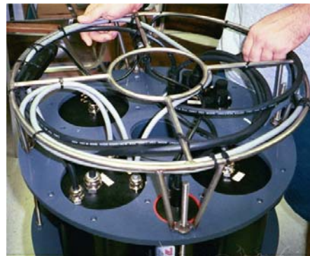
Fig. 8: Underside of AUV, with spacer plate and skid cage shown
