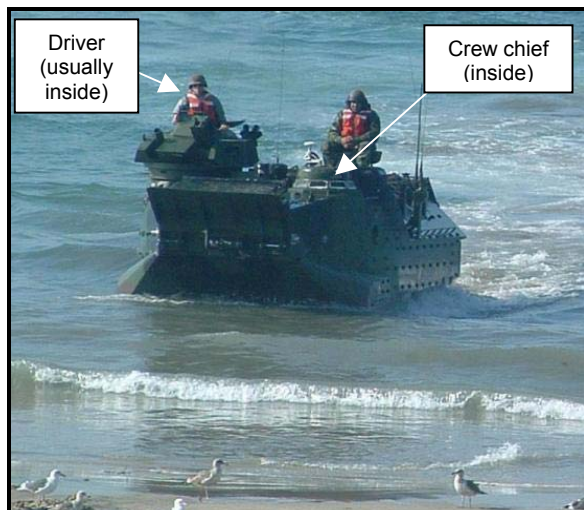
Fig. 2. Primary crew locations on an AAV.
