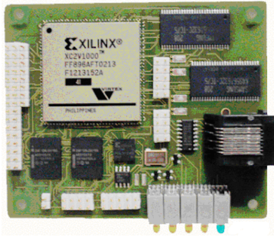
Fig. 11. The prototype board for the hardware correlator. Physical size is 90 mm x 70 mm.
