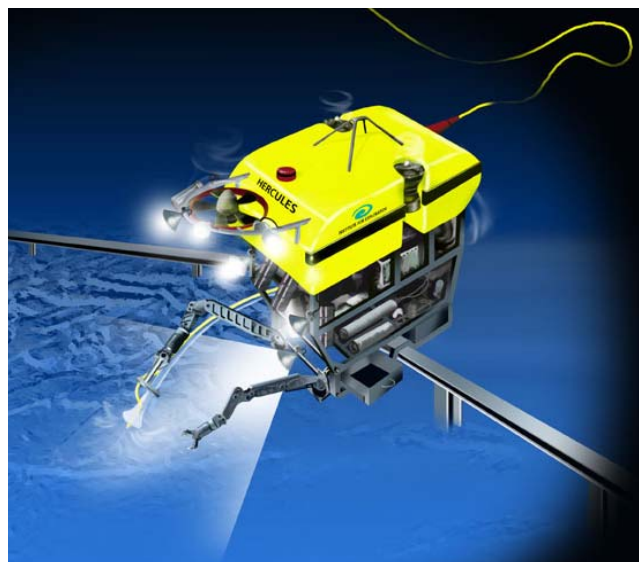
Fig. 9. Artist's sketch of the ROV Hercules , coupled to the gantry frame, excavating the sediment within and around an ancient shipwreck.
