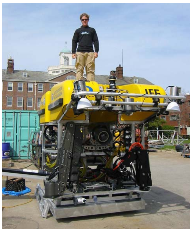
Fig. 8. Excavation ROV Hercules , viewed from the front, being prepared for dock trials in Woods Hole. The high-definition video camera is mounted on a pan-tilt unit in the center. Hydraulic manipulators are on each front side corner and can swing aft and down.
