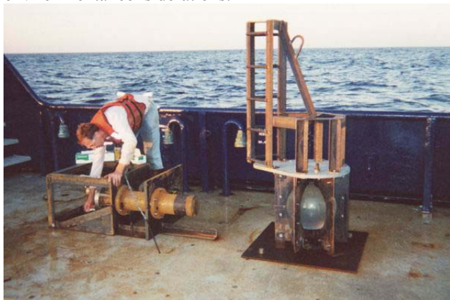
Fig. 1. Cylindrical and spherical imploder configurations
