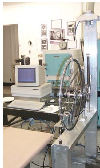
Fig. 1. The apparatus for studying the friction coefficient
