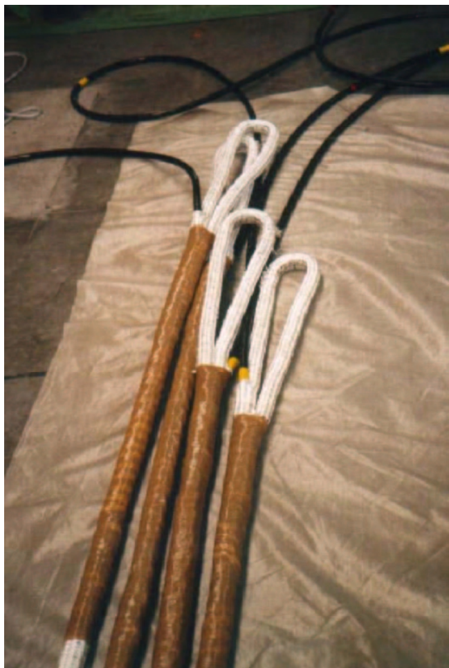
Fig 12; Transducer Built into Rope
