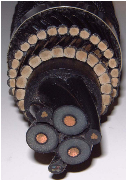
Fig.11 Cross-Section of KAIKO-No.1 Cable
