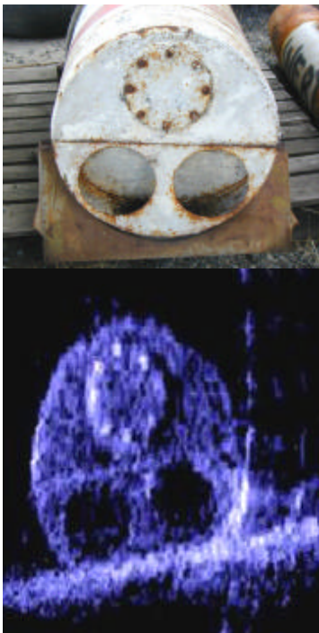
Fig. 10. Photograph and a DIDSON image of a mine shape.
