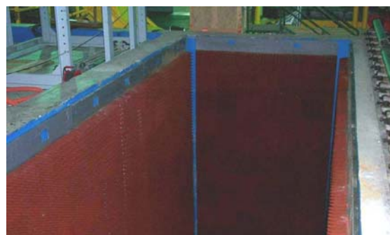
Fig. 1 Photograph of the anechoic tank at KRISO/KORDI before the construction of the test room over the tank (dimensions: 914cm x 282cm x 500cm)
