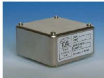
Fig. 7. RMO rubidium oscillator.
