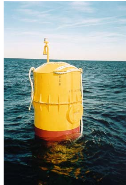
Figure 6: Initial feed buoy deployed at the site.
