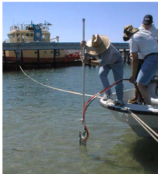
Fig. 10. Deployment of the Trident probe from a small boat using the push rod and air hammer.
