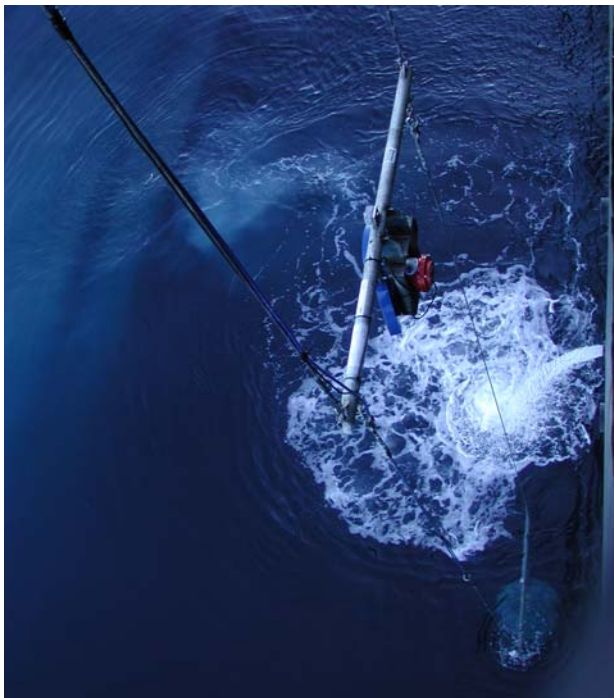
Fig. 3. The H-ADCP is suspended above down-looking ADCP and lowered via the dual-winch system.
