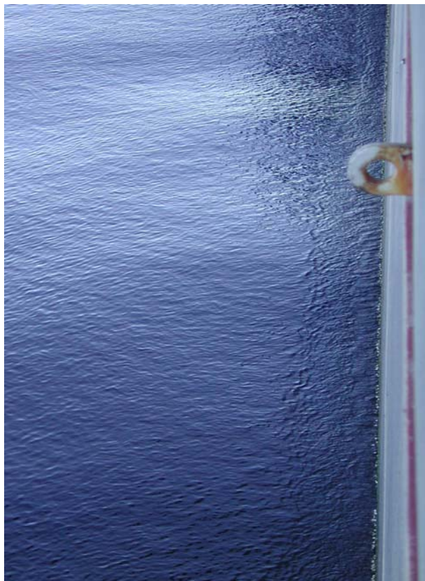
Fig. 5. Capillary wave structure near the hull of the CR Luigs shows the direct input of energy to the water.
