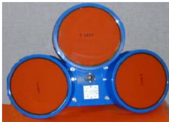
Fig. 1. Long Range 300 kHz Horizontal ADCP
