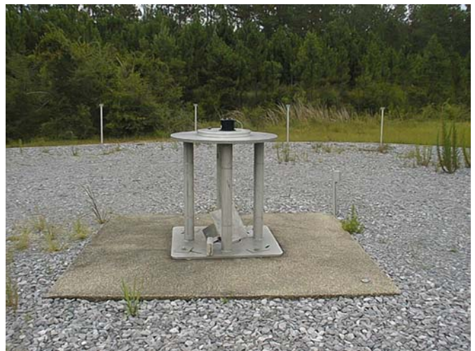
Fig. 5. The platform that supports the sensors at the center of the "compass rose."
