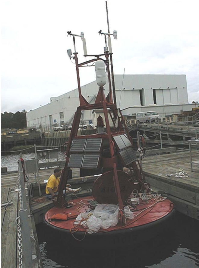
Fig. 2. A 3-meter discus-hull buoy undergoing a “buoy spin” magnetic sensor test.
