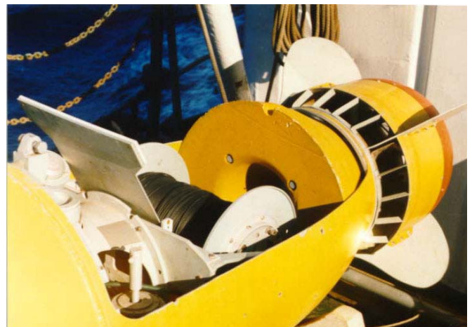
Fig.3. Reel with fiber optical cable in the stern part of TSL.
