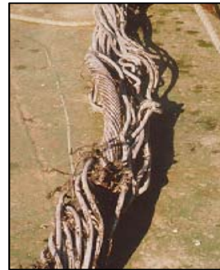
Fig. 2 Damaged shallow water cable after contact with fishing tackle
