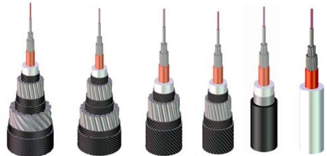
Fig.4 .Range of medium voltage telecommunication cables from deepwater on the right to shallow water on the left
