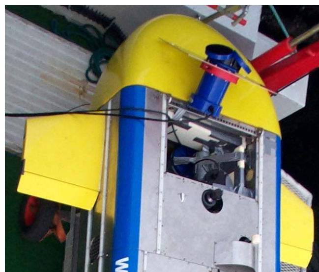
Fig. 3 The M-150 AUV with two ADCP and the CTD sticking out of the hull. The NORTEK ADCP is on top of the AUV, while the RDI unit can be seen in the payload bay.
