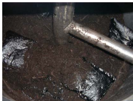
Fig. 8 Compost and SBS with oil in the tank
