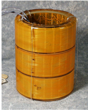
Fig. 3 Three encapsulated free-flooded ceramic rings as a stack with 0.1 inch spacing.
