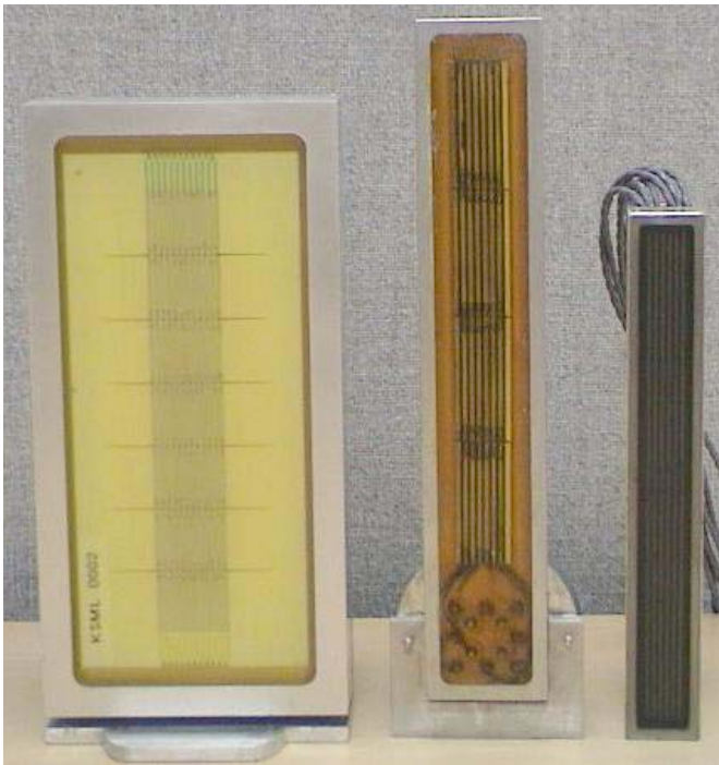
Fig. 5. The three arrays used to explore the effects of crosstalk. Array A is on the left, array B is in the middle, and array C is on the right.
