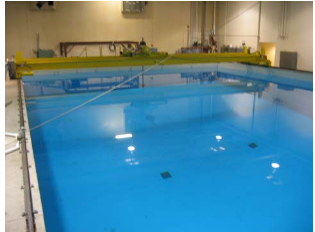
Figure 1. The hardware for the positioning system: X-Y bridge-carriage, and the Yuasa rotation table and controller. The tank has a 40' span, the rails run along the 60' length, and the tank has 20' of water.
