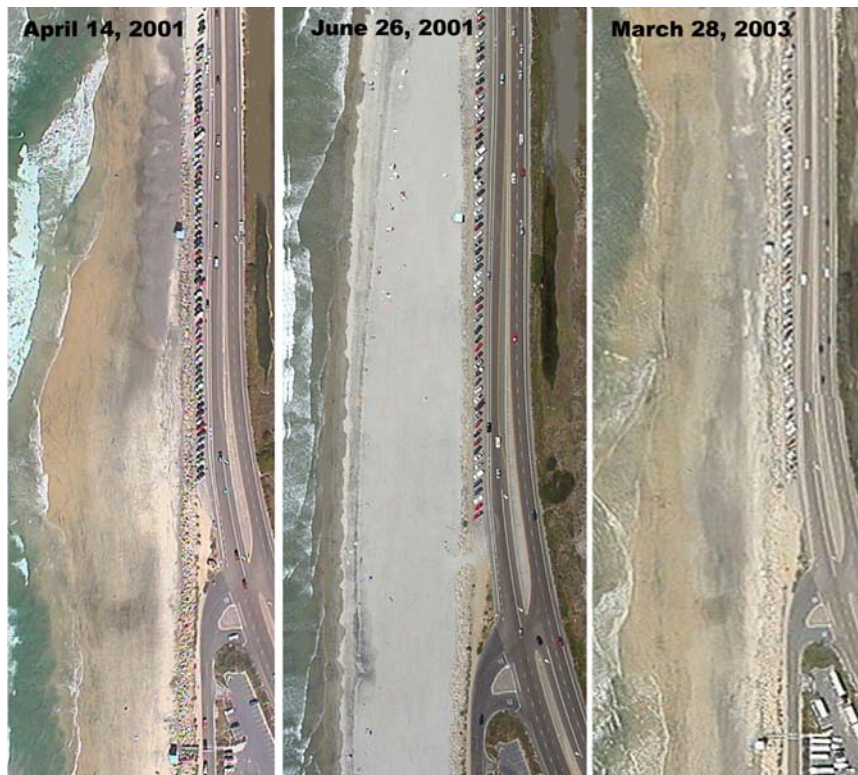
Fig. 3. Photograph showing Torrey Pines Beach before and after 260,000 yd 3 sand placement on the beach in late April 2001.
