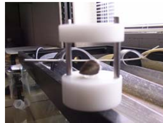
Figure 10: Jig for gluing screws and magnets to clams
