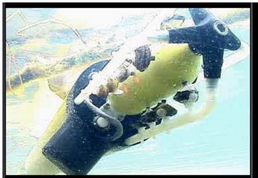
Figure 12: Open water testing. Clams are siphoning with mantle extended; LEDs are on
