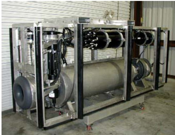
Fig. 1: HIDEX II Profiling Package (skid)
