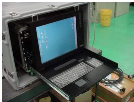
Fig. 9: Topside Computer & Telemetry Console
