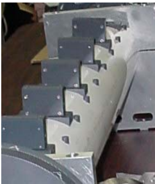
Fig. 3: Detection chamber with fiber-optic penetrators
