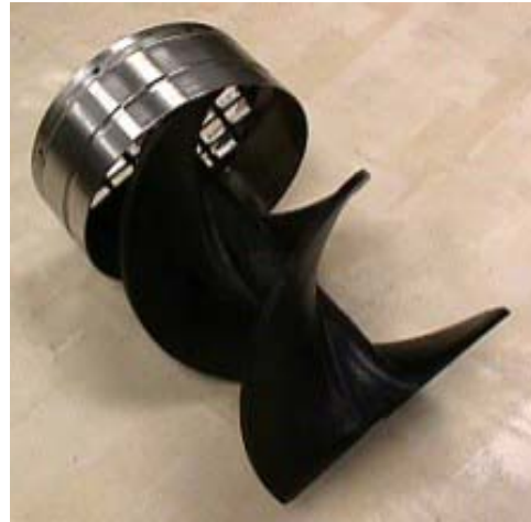
Fig. 2: Helical light baffle with excitation grid
