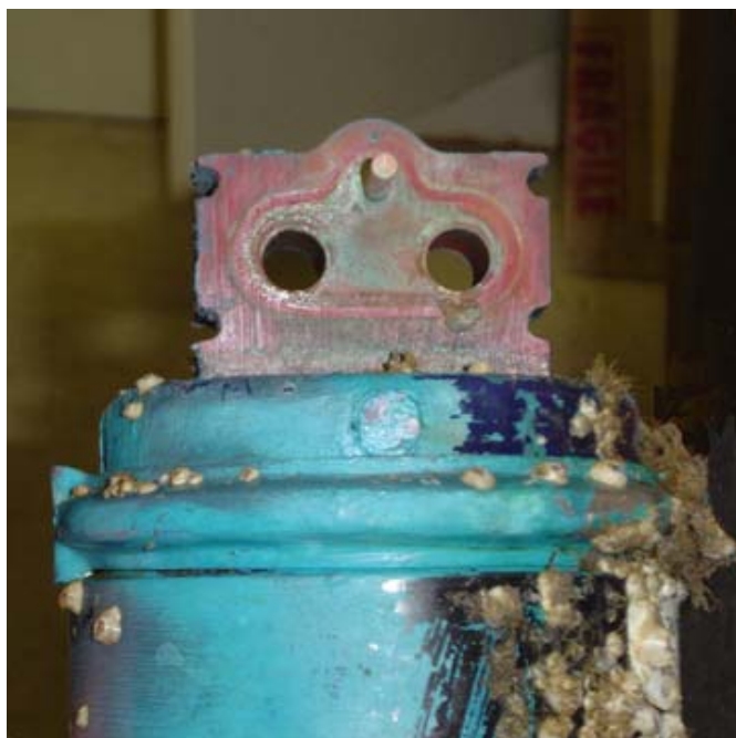
Fig 5 View of the inside tubes of the NXIC sensor after deployment - no fouling
