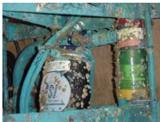
Fig 4 External Views of NXIC sensor and current meter after retrieval. Note that the antifouling paint, fouling has attached to the surfaces.
