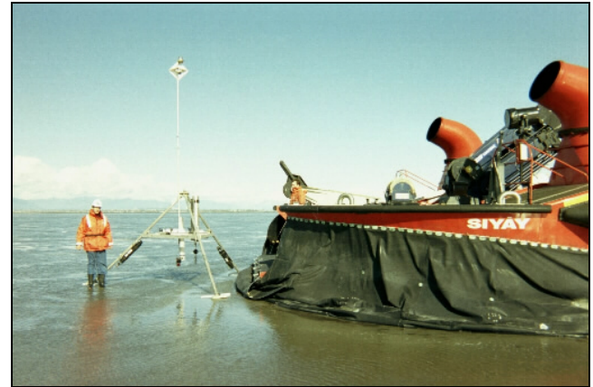
Fig. 4. Deployment of Norton on Roberts Bank March 23, 2003 using the Canadian Coast Guard Hovercraft Siyay . A radar reflector and flashing light were mounted on a pole above the tripod.
