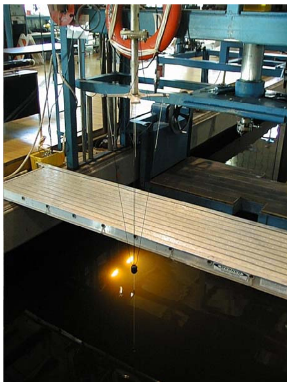
Fig. 2. Vector sensor tethered from rotation test shaft
