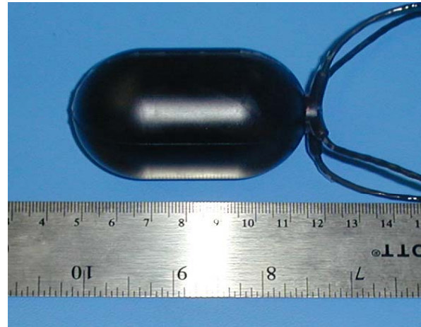
Fig. 1. Finished vector sensor and was located 2 meters from the sound source. A gated pulse method was used to obtain the data.
