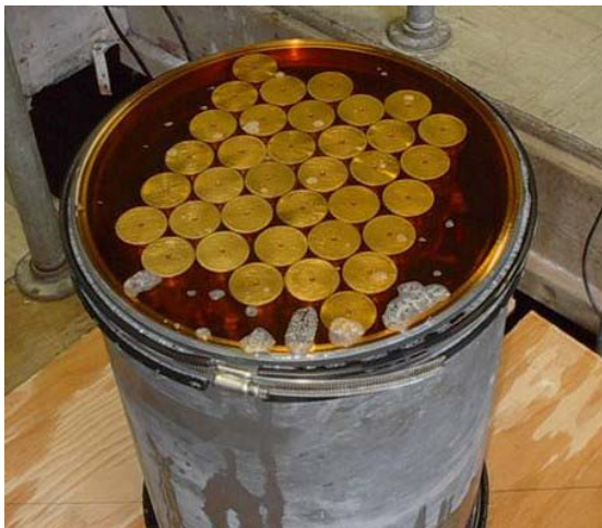
FIG. 13 Thirty-six element staggered array.
