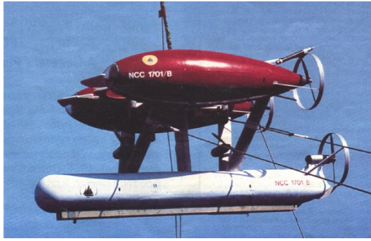
Fig. 4. The Autonomous Benthic Explorer (ABE) vehicle.
