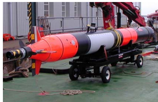
Fig. 1. The UUV mine reconnaissance demonstrator
