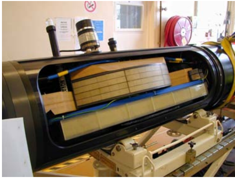
Fig. 2. Configuration of side-looking sonar transmitter (curved) and hydrophone array
