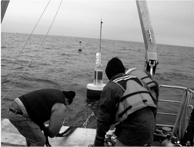
Fig. 9. The buoy has just been launched, and the elastic tethers are being paid out over the stern by hand. The remaining components are deployed over the stern by hand down to the anchor.
