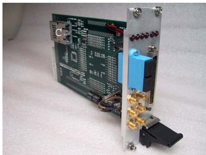
Fig. 4. Telemetry interface, Front Panel and Solder Side
