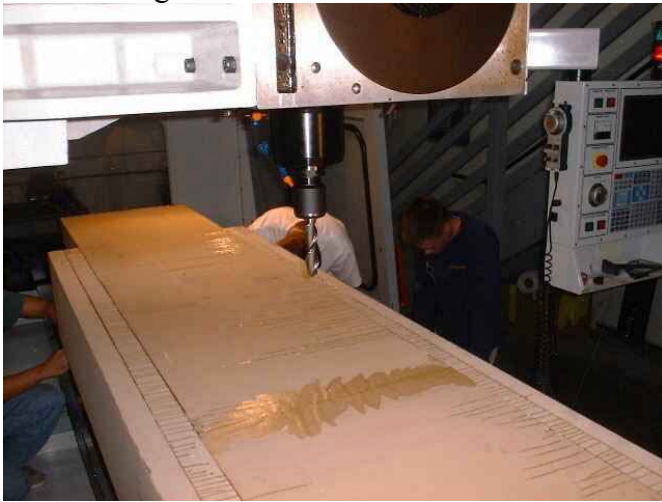
Fig 1- CNC Machining of mold at HAAS Machining in Oxnard, California
