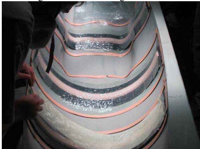
Fig. 3 Creating the Strengthening Ribs
