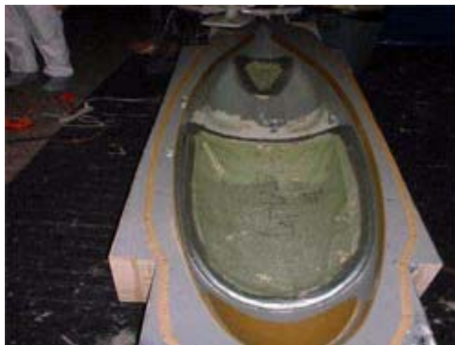
Fig. 4 Pilot and drive-train hatches prior to lay up of top half.
