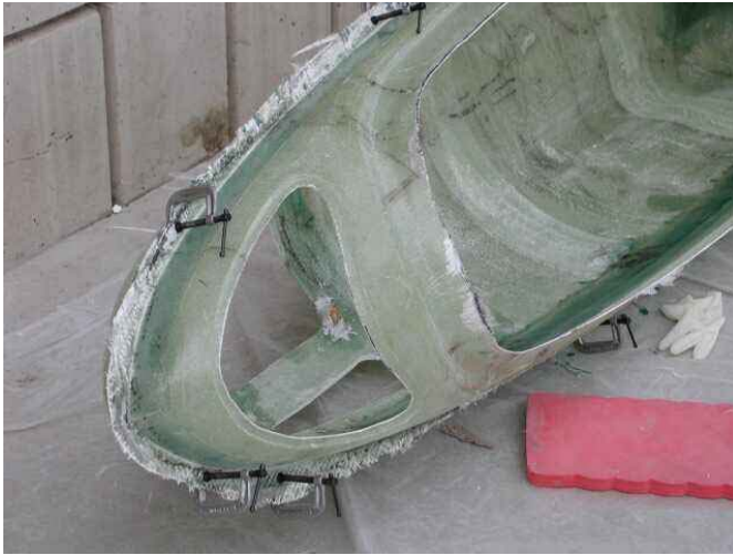
Fig. 2 Joining the two halves. With the two halves held together by C-clamps, 4" wide strips of composite are run lengthwise along the hull after removing the excess flange material.
