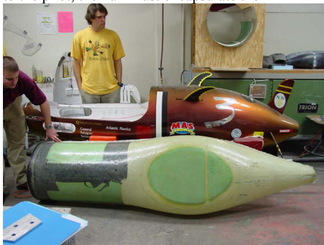
Fig. 3. Closed-cell foam (green) and carbon reinforcement (black) visible
