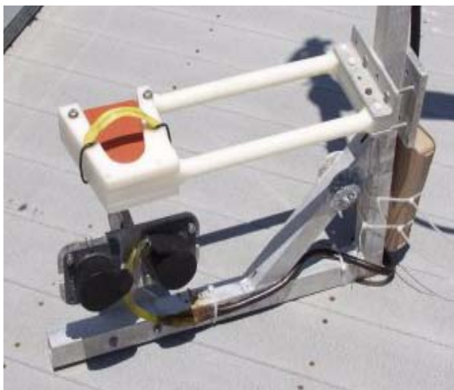
Fig. 3. The bite plate stationing device and the binaural receiver mounted directly below and in line with the animal's MRA. The animal is trained to bite on the soft rubber insert (fitted to its rostrum shape) and hold during echolocation.
