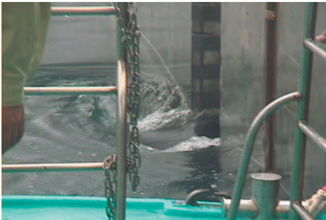
Fig. 15. Strong cyclic flow caused by the slit.
