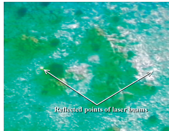
Fig. 17. Undetectable reflected points of laser beams on the caisson.
